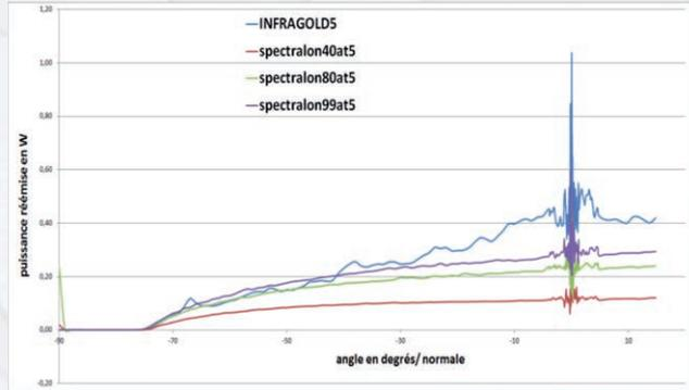
Figure 4 : BRDF measured on PROMATSOL's standards
