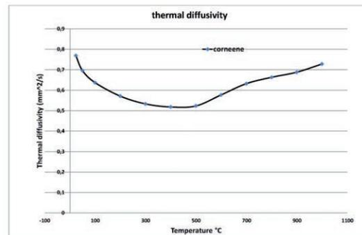
Figure 2 : Thermal diffusivity of Cornéenne sample
