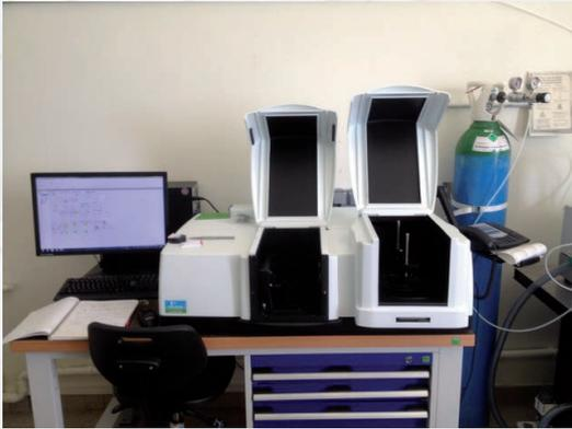
Figure 7 : Lambda 950 fitted with the TAMS accessory
