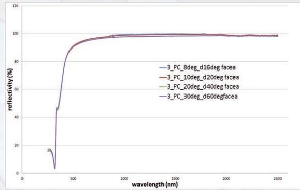
Figure 8 : Reflectivity of « miroir\_3PC » face A, face B with and without specular component
