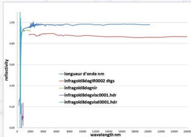
Figure 6: Hemispheric Reflectivity of a standard compared to its measurement with the SOC100HDR
