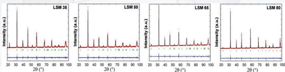
Figure 7 : LeBail fits of X-ray diffraction data collected for LSM perovskites. Experimental (red), calculated (black) and difference (blue) curves
