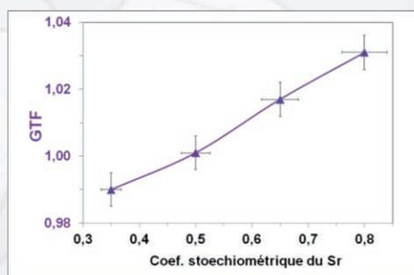
Figure 9 : Calculated Goldschmidt Tolerance Factor (GTF) of the LSM compounds.
