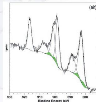
Figure 5 : Ce 3d3/2,5/2 XP-spectra collected for  $\text{La}_{0.8}\text{Ce}_{1.2}\text{Zr}_2\text{O}_{7.6}$  compounds elaborated under air
