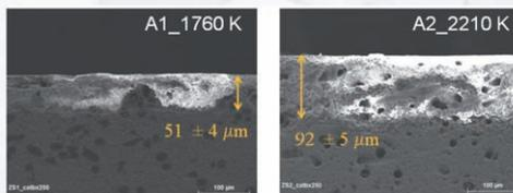
Figure 13 : SEM cross-section collected for samples A1 (1760 K) and A2 (2210 K).
