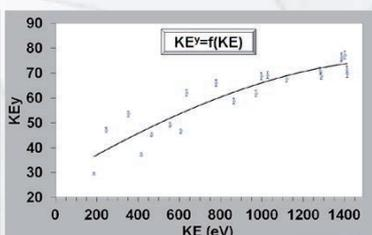
Figure 2 : Instrumental function of spectrometer (KEY) v.s. kinetic energy of the photoelectrons (EK).
