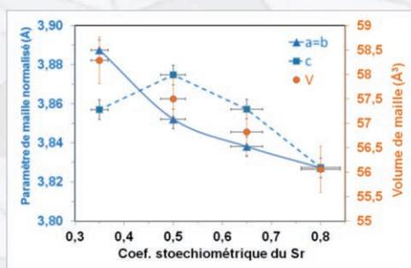
Figure 8 : Crystallographic data calculated from LeBail fits. The cell parameters were normalized from ideal cubic perovskite structure.
