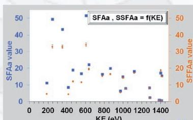
Figure 1 : Calculated (SFFAa) and theoretical (SFAa) sensitive factors v.s. kinetic energy of the photoelectrons (EK).
