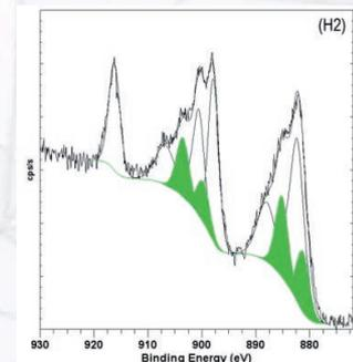
Figure 6 : Ce 3d3/2,5/2 XP-spectra collected for  $\text{La}_{0.8}\text{Ce}_{1.2}\text{Zr}_2\text{O}_{7.6}$  compounds elaborated under  $\text{H}_2$
