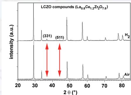
Figure 4 : Diffractograms collected for  $\text{La}_{0.8}\text{Ce}_{1.2}\text{Zr}_2\text{O}_{7.6}$  compounds elaborated under  $\text{H}_2$  and air.
