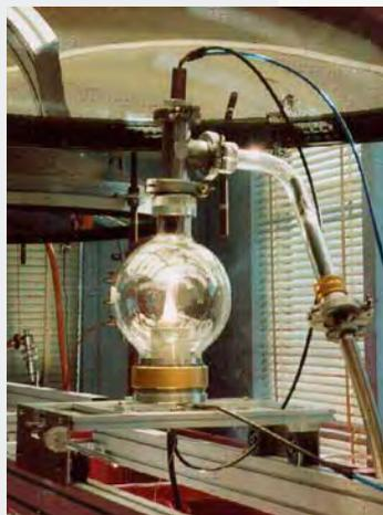
Figure 11: Solar reactor Heliotron used to prepare nanopowders by SPVD.
