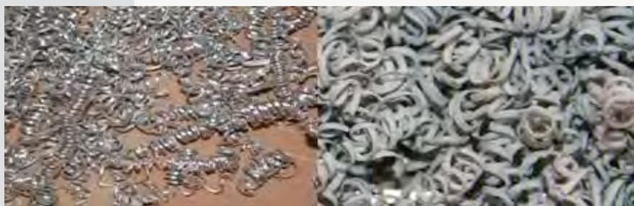
Fig. 13: Picture of metallic chips with and without coated TiO<sub>2</sub>.
