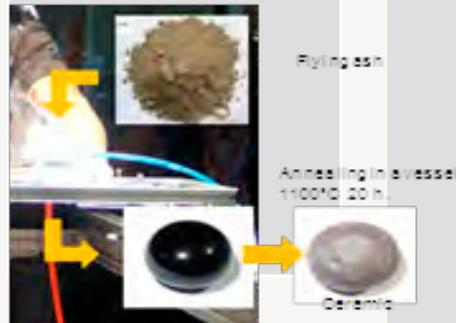
Fig. 2: Vitrification of fly ash under concentrated solar flux. Ceramic is obtained by annealing.
