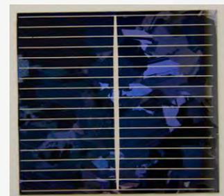
Figure 16: Photography of a 5x5 cm<sup>2</sup> solar cell with an AP-PECVD antireflective and passivating coating.
