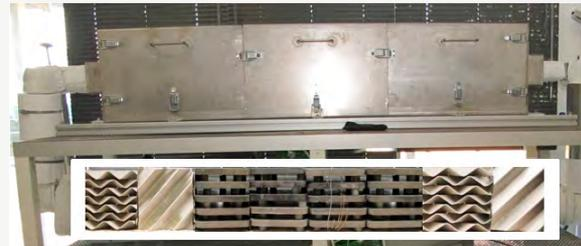
Figure 4: Set up for storage/destorage of energy with recycled wastes (900 –300°C). View of the internal air pipe equipped with static mixers and ceramic plates.
