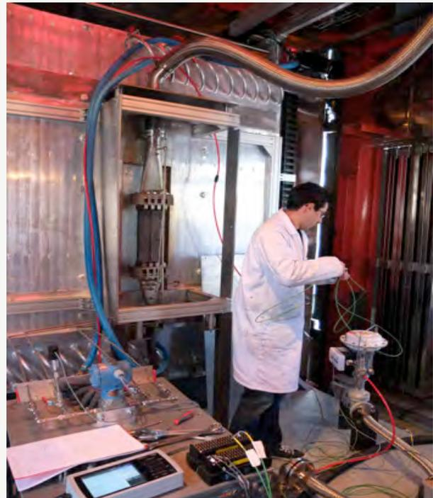
Figure 3. Testing of a ceramic module at the focus of the 1MW solar furnace
