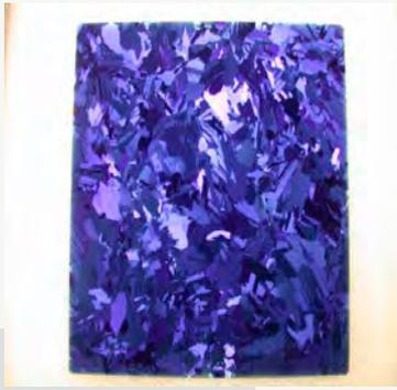
Figure 13: LF PACVD a-SiCNH film coated on a polycrystalline Si square wafer
