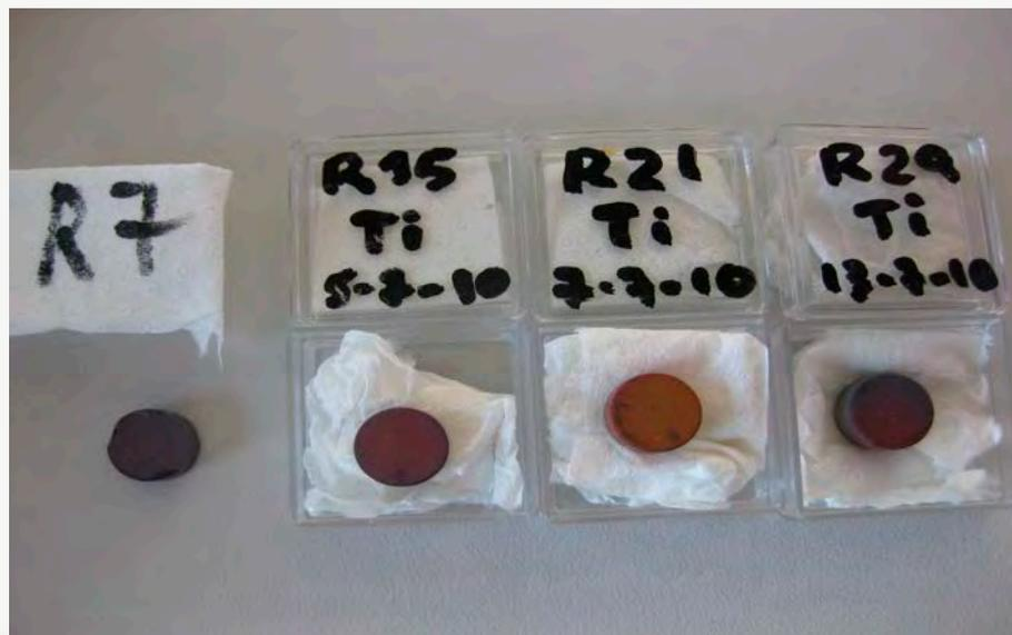
Figure 16: Photos of the samples of the Titanium series (R7 set-up A no filter, R15 set-up B no filter, R21 set-up B Blue sky filter and R29 set-up B Medium yellow filter)
