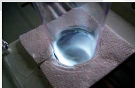
Figure 9 : MESOX solar reactor at the focus of the 5 kW solar furnace and image of the CO<sub>2</sub> plasma
