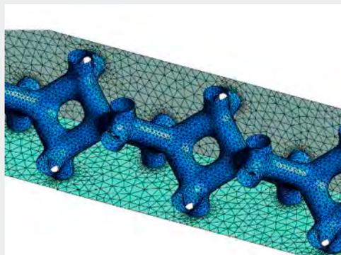
Figure 5. Wall and fluid meshes used (refined near wall)
