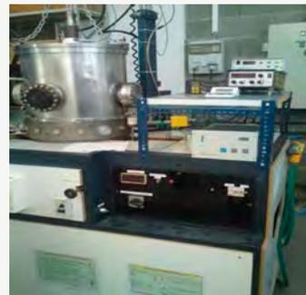
**Figure 6:** Rf-magnetron sputtering process allowing making nanostructured thin films.
