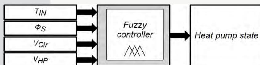
Figure 4. Structure of the proposed fuzzy controller.
