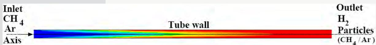
Figure 9. Contour plot of flow temperature in the tubular reactor for methane decomposition.
