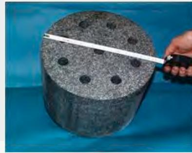
Fig. 6: PCM/ENG composite for the thermal protection of solar receiver (ANR Solstock).
