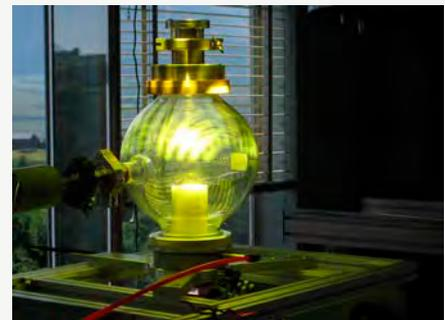
Figure 15: Reactor appearance during experiments (Sky blue and Medium yellow filters)
