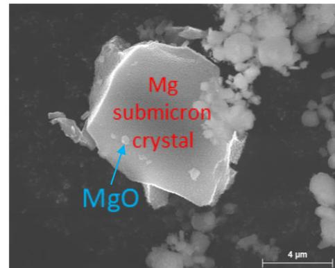
Granulometry: agglomerates of sub-micron Mg particles and crystals,  $D_{90}$  of 100  $\mu\text{m}$  (40% are < 10  $\mu\text{m}$ ).
