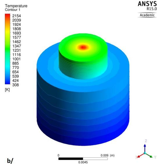
Temperature distribution on the Sol@rmet reactor and the surface of the C/oxide pellet
