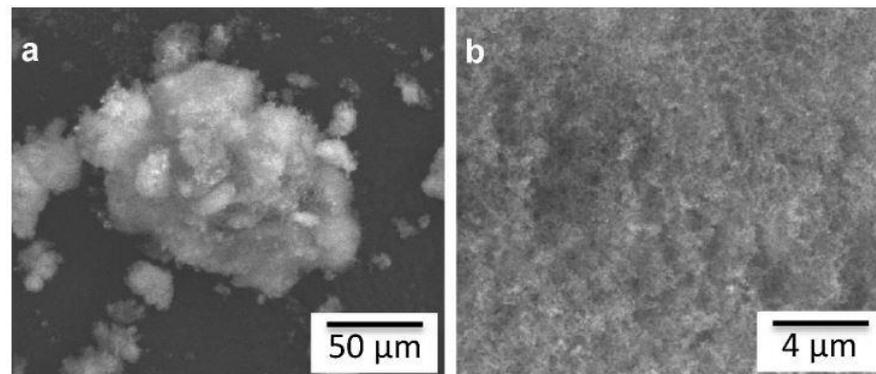
**Granulometry:** agglomerates of nano- and micro-sized Al particles,  $D_{90}$  of 3  $\mu\text{m}$  (50% are < 50 nm).
