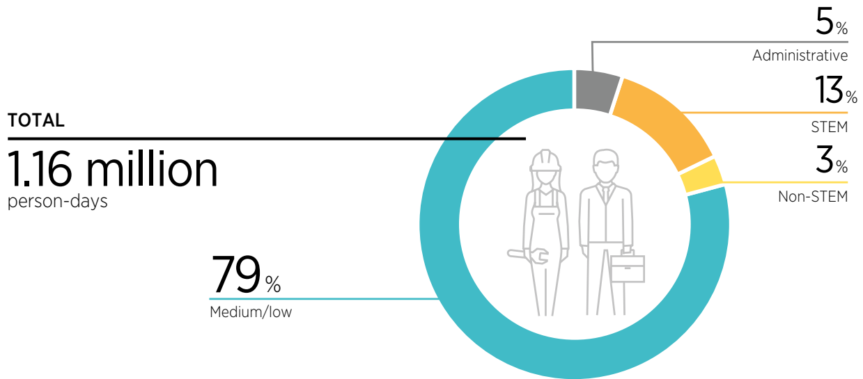
Figure 7 ■ Distribution of the skills required for developing a 100 MW CSP plant with ten-hour TES capacity
