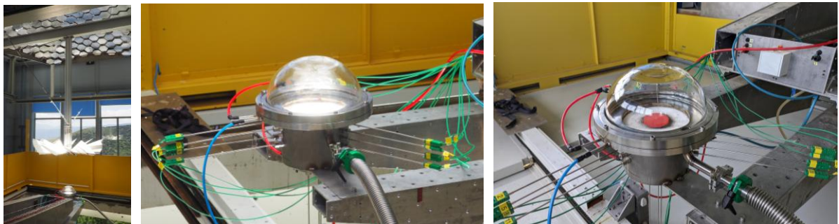
Figure 2 : Experimental solar TPV setup operating at the 6-kW solar furnace in PROMES.
